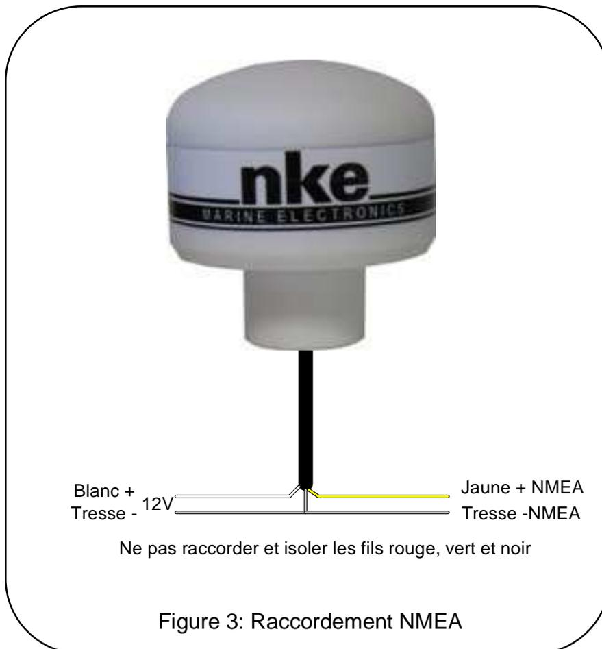
Figure 3: Raccordement NMEA
