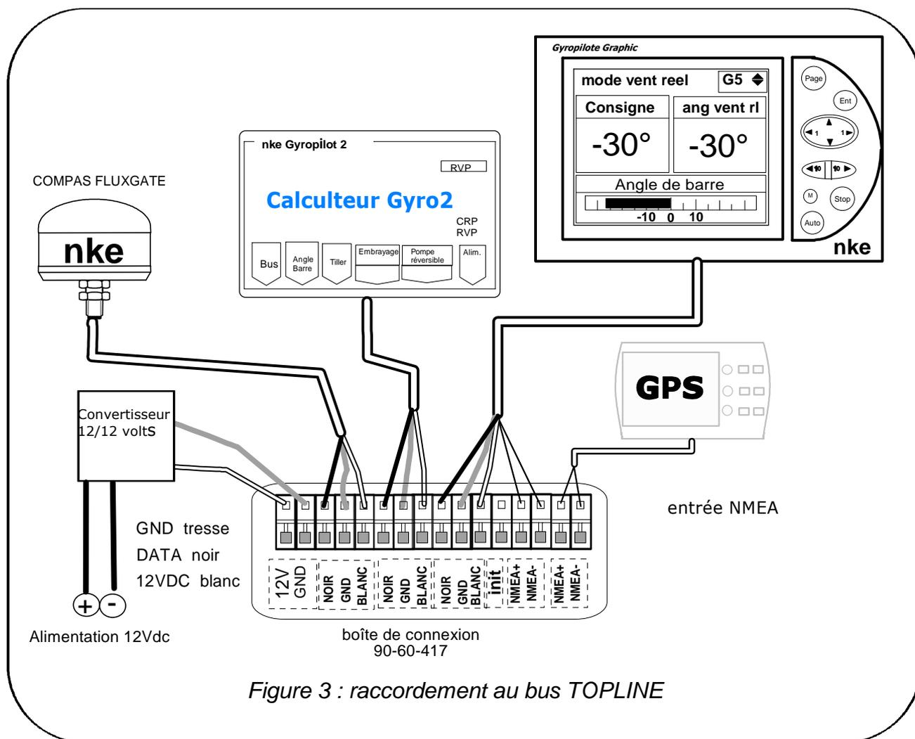
Figure 3 : raccordement au bus **TOPLINE**
