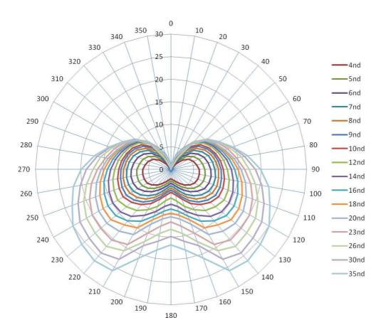
The diagram shows the target boat speed against wind speed and wind angle.
