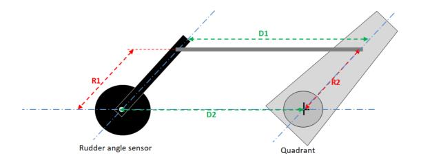
Picture1: installation of a nke rotary rudder angle sensor
