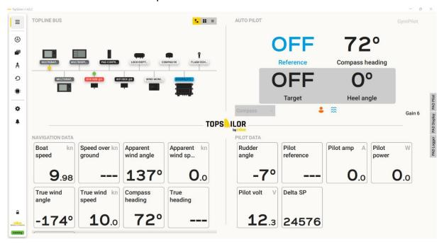
At the top left is a model of the system including all the instruments used, with a display of names and addresses, as well as a color code (refer to §Architect). It is possible to select an instrument to open its information page.
