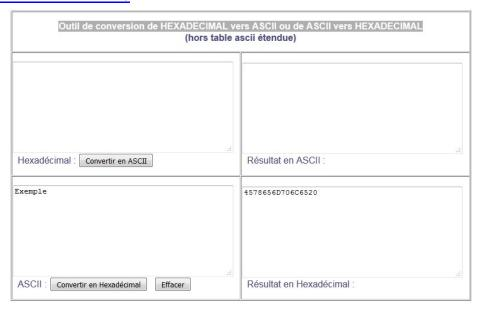
In this example, we use the website to convert the text "Example" into hexadecimal code. The values integrate a pack of two letters. In this case "Ex" is interpreted as the hexadecimal code "4578".
