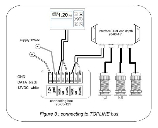
If you reduce the length of the bus cable 90-60-460, strip and galvanise the wires before connecting them inside the terminal box.
