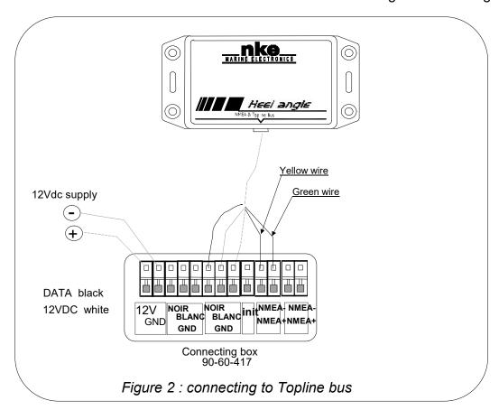
If you reduce the length of the bus cable, strip and galvanise the wires before connecting them inside the terminal box.
