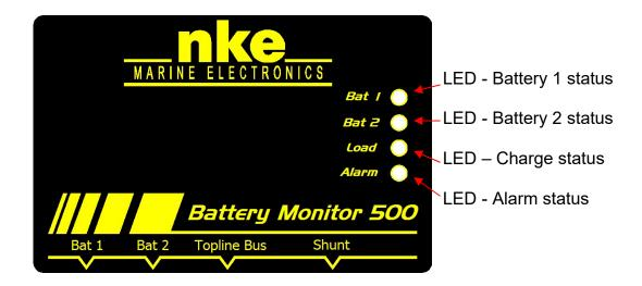
LED *Bat 1*: Indicates the measured voltage on battery #1. LED is green when the measured voltage is > 11.6 V (or 23.2 V), and red when the measured voltage is < 11.6 V (or 23.2 V). LED is off if the *Battery Monitor 500* is not connected to the battery #1
