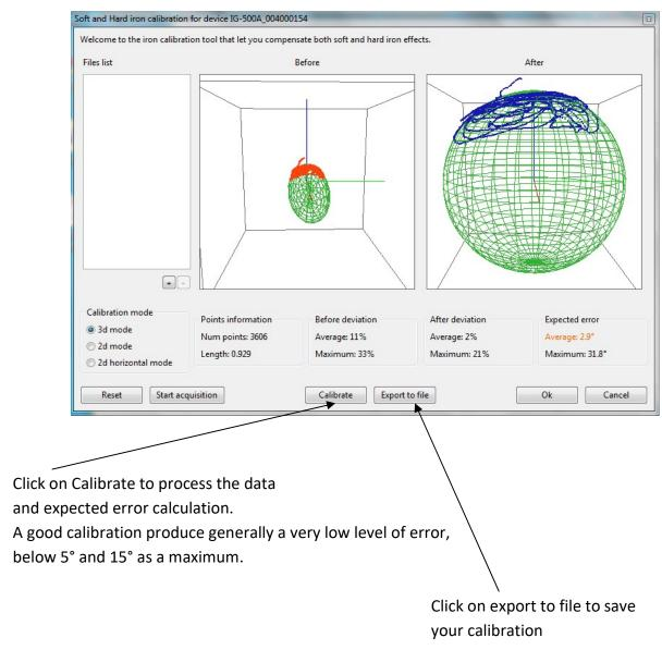
One can make several calibrations and save them. They can further be complied in one single deviation correction saved in the 3D Sensor. This gives the possibility to make calibrations in several orientations.
