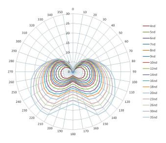
The diagram shows the target boat speed against wind speed and wind angle. As shown on the picture below, a target boat speed upwind is determined with a line perpendicular to the boat speed axis and tangential to the highest point of the curve.
