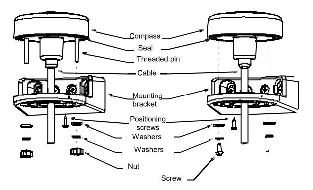
Pass the connector of the compass through the seal. Connect the cable to the compass. Insert the seal onto the compass so as to match the mounting holes between the compass and the seal.
