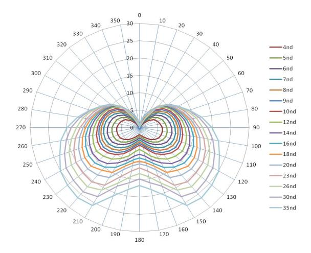
The diagram shows the target boat speed against wind speed and wind angle.
