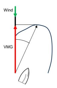
VMG = boat speed Xcosine (True Wind Angle)
