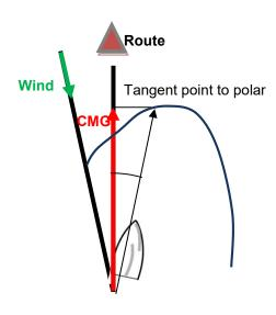
CMG = Boat speed \* cosine (Heading - Marks bearing)
