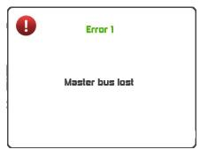
The "master" display is unplugged or out of order. This can be solved by replacing the "master" display by another one. (Refer to "Topline addresses" section).
