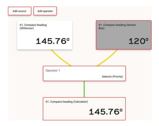
The operator is of selector type and is in priority mode. This means it will feed the output data with the first valid data source starting from the left. In our case, the heading stemming from the 3D Sensor HR is selected.
