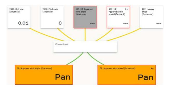
Straight away, we observe that the corrected apparent wind angle and speed channels are in PAN, and this is due to the fact that there is no raw wind data at the calculation input. This is a Processor calculation, and as we have seen previously, these calculations cannot be modified by the user. The latter can only input the sources.
