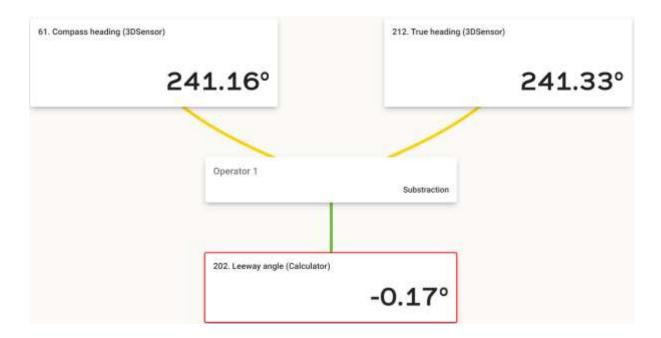
In the "apparent wind correction" calculation, we check the source for the "Leeway angle" data type. It must use the "Calculator" source. Notice that our leeway angle is correctly injected into the de-noised apparent wind calculation.
