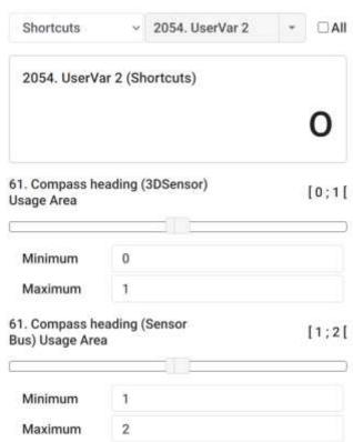
**NOTE**: We will need to use a Selector (variable) to select per hysteresis variable. To create a hysteresis, leave a margin between the different thresholds, which corresponds to the hysteresis, in the following case, a trigger threshold of 10 units:
