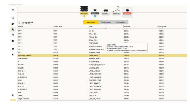
**NOTE**: By configuring the "Config NMEA" register (formerly called "tracker") in "Processor X Mode" mode, the transmission speed of the compass 9X's NMEA output is set to 115,200 baud. The "Baudrate\_NMEA" register value is not used.
