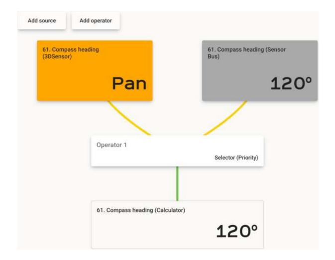
There is no more data from the "3DSensor" source, hence the display of the "pan" message. Observe that the selector is now feeding the "Compass heading (Calculator)" output data with the heading data from the compass 9X.
