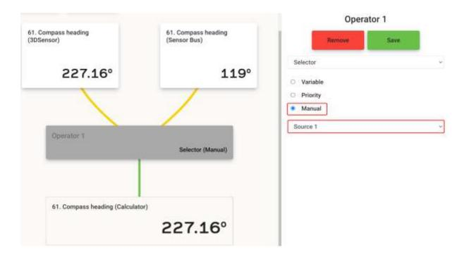
In our case, we want to use the 3D Sensor HR as the main source, meaning we manually set the selector on source 1.
