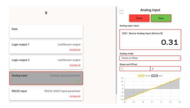
In the case above, the analog input was connected to a signal between OV and 5V.
