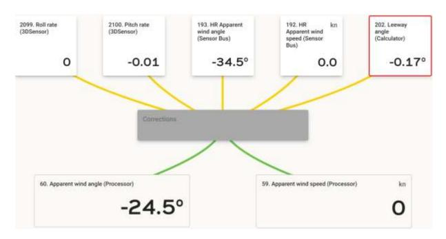
The operator also makes it possible to run additions, multiplications, divisions (including options with and without modulo), along with fixing values. You can use these operators with the same reasoning as that explained above.
