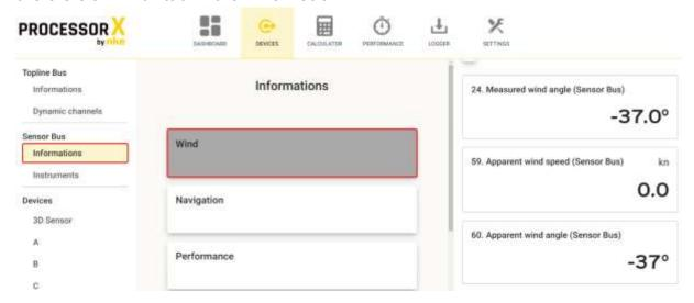
**NOTE1**: the Processor X must imperatively be set to address 1 on this bus. The Processor address configuration is not available on the Sensor bus.
