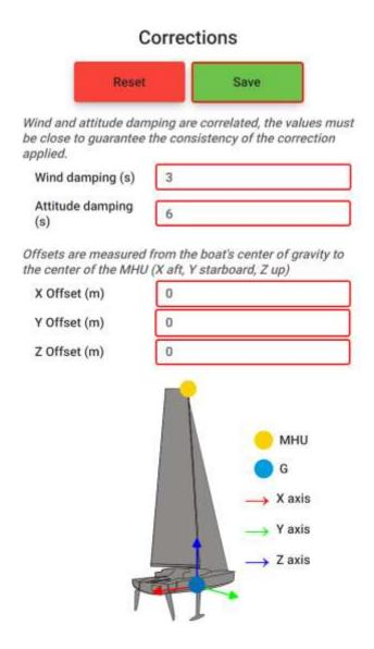
The filtering parameters are available along with the "Wind damping" and "Attitude damping" fields.
