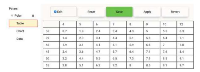
While editing, the "Reset" button makes it possible to load the default table. The "Save" button makes it possible to save the table and relaunch the performance calculations with the new table. The "Apply" button is similar to the "Save", except that it enables you to continue editing the table. The "Revert" button makes it possible to cancel an unsaved entry.
